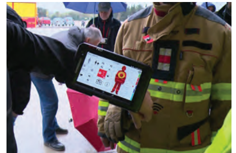
The prototypes can gather sensory, biometric and localisation data and relay them to a visual interface in the hands of a commanding officer.
